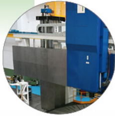
Continuous W axis with mechanical locking system for high rigid turning
