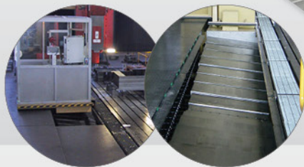
Automatic telescopic walkable bridge for operator operations
