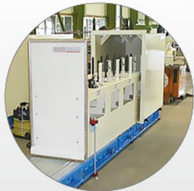
Fully Automatic accessory change and travelling robot for tools
