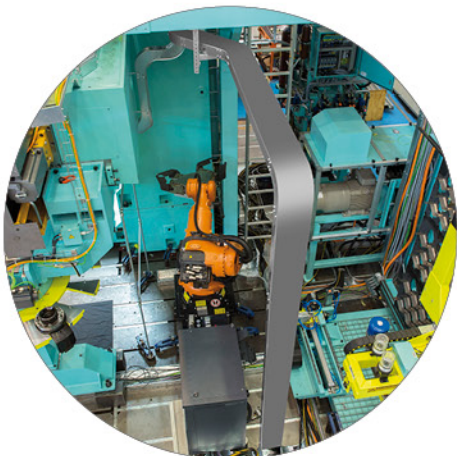
Tool Management System: shuttle to handle thousands of tools connecting machine tool magazines
