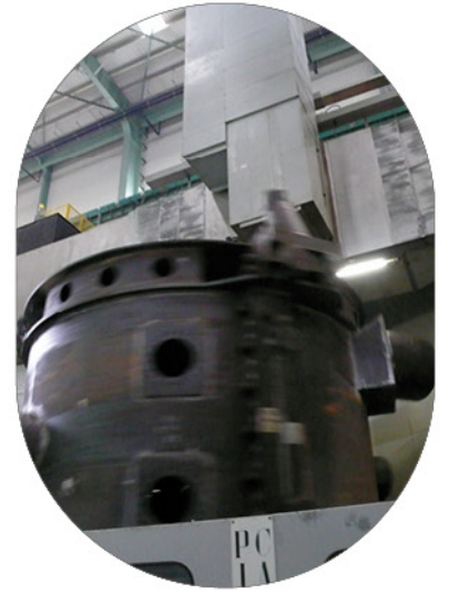
Special T slot cutting package for turbines applications (movable axis toolholders, minimum boring size, rigidity at extreme Z axis stroke, dampening sensor and special software package)
