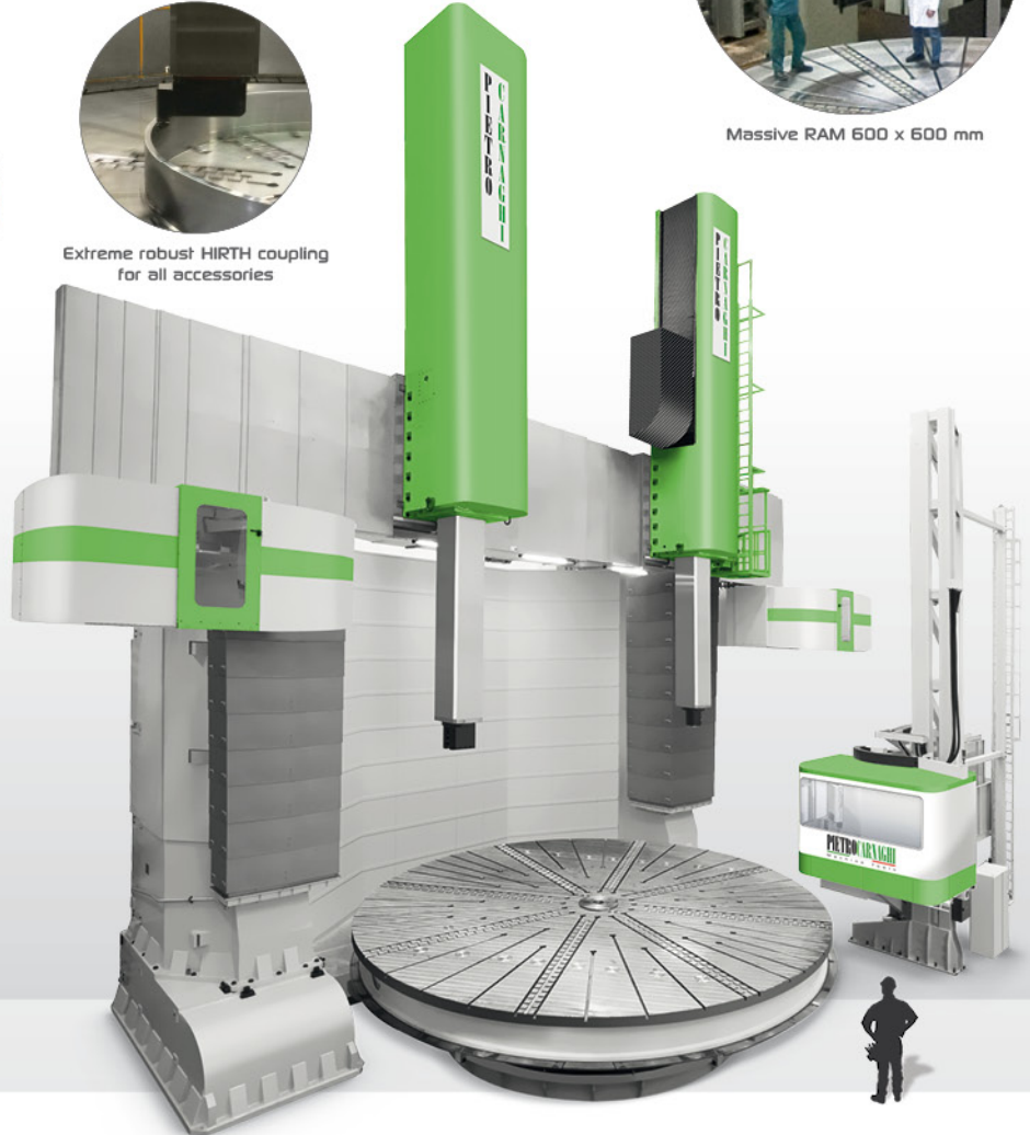
Continuous W axis with mechanical locking system for high rigid turning
