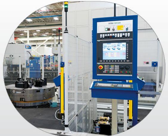
FMS production software studied to optimize the scheduling of part programs, tool management, part probing, calibrations and feeding in the workpieces.
