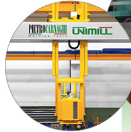
Separate Bridge with fully movable operator platform in machining area
